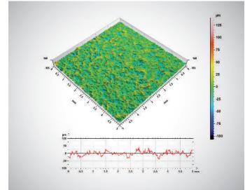
Rz: 74 μm – Rmax: 79 μm – Pc: 28 inches > Homogeneous surface profile thanks to narrow hardness range
