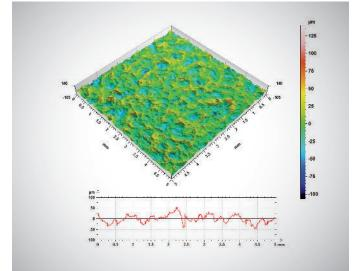
Rz: 77 μm – Rmax: 89 μm – Pc: 20,5 inches > Heterogeneous surface profile
