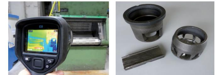
Wear monitoring and blast pattern check using WA CAM
