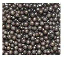
Figure 2: Low-Carbon Cast Steel Shot
