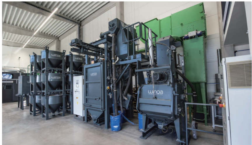
Airblast, Tumblast and Spinner hanger blast machines for training and trials
