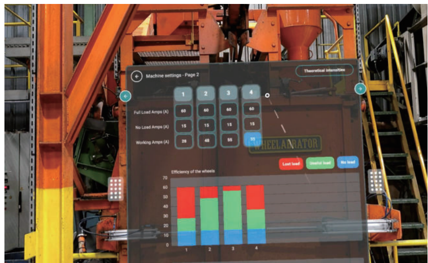
Augmented Reality Efficiency Analysis of a Blast Machine
