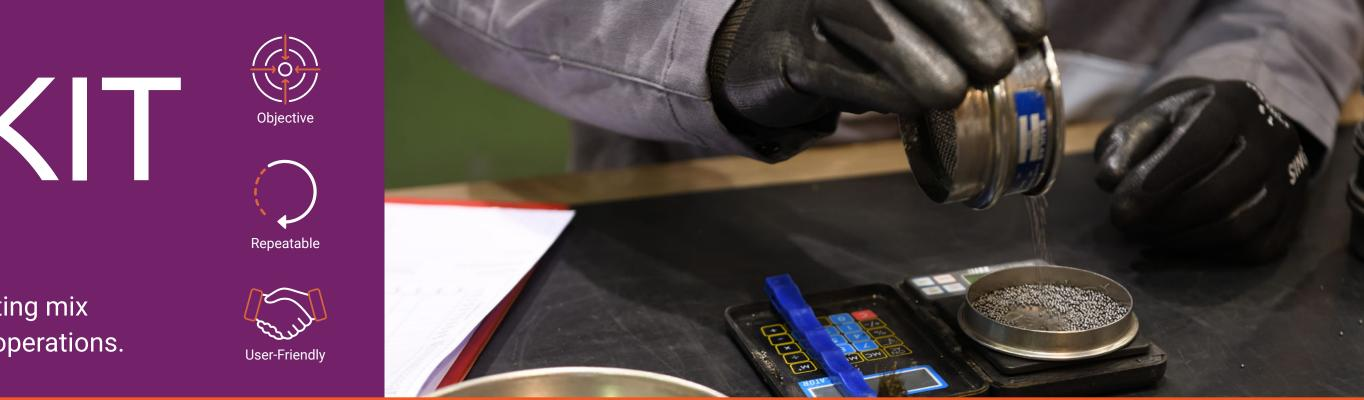
• The **BLAST CHECK kit** is an easy-to-use tool designed for inspecting the active operating mix used in blasting operations. All you need to do is collect a representative sample from the air washer (at the shot curtain) and sieve the sample using the filter set included in the kit case.
